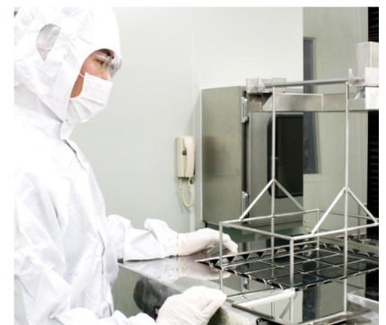
Ultrasonic Cleaning (Class 1000 Clean Room)
